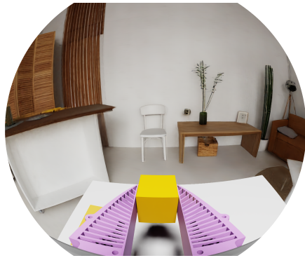
Figure 12: Fisheye view of UMI pick-and-place manipulation with a rigid cube.
